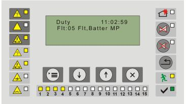
For any fault condition in the remote fire control panels, indicator pos. 4 (Fault) illuminates in flashing yellow light. Depending on the specific fault, the following indicators are illuminated too:
